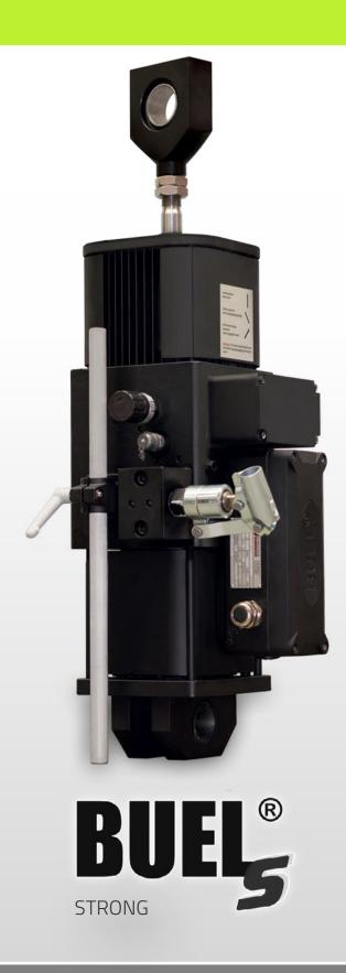
The BUEL® Model S is a new family member of the DELLNER BUBENZER brand BUEL®. It is designed for wheel brakes on rail mounted cranes, where high pulling forces for mechanical wheel brakes are required. The patented cylinder system generates pulling forces up to 40.000 N. It has a robust, but also compact design for rough environmental conditions. **Our experts will assist you to find your best solution with BUEL®**.
