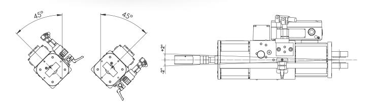
**Installation positions**BUEL® Model S units are preferably operated in horizontal position.
