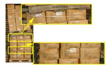
When stacking loaded pallets on top of each other, it may be advisable to use intermediate layers to distribute the load. The maximum weight specified in section 9 must not be exceeded.
